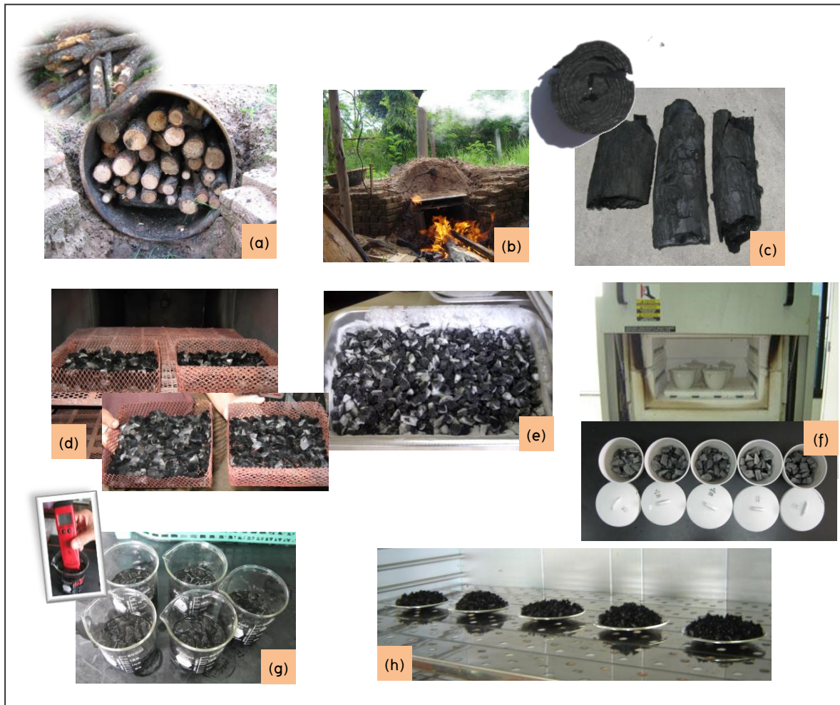
Figure 1 Methods of activated carbon preparation from Pinus caribaea
