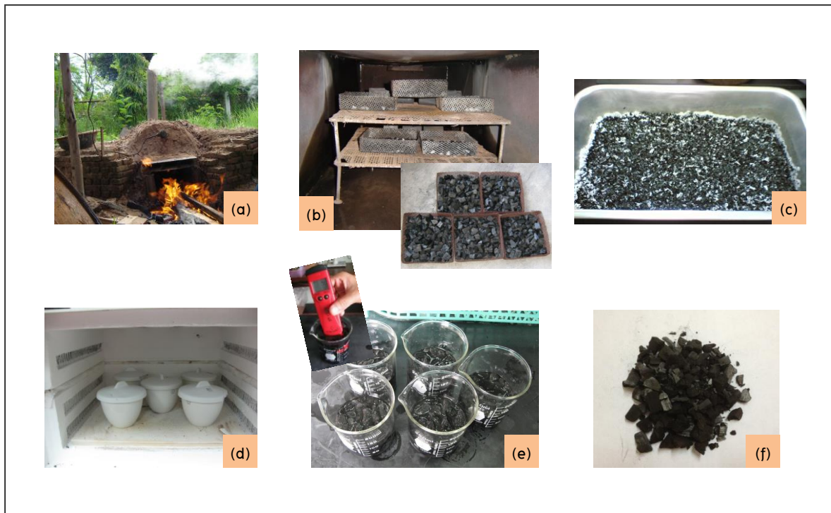
Figure 2 Methods of activated carbon preparation from Acacia mangium preparation
